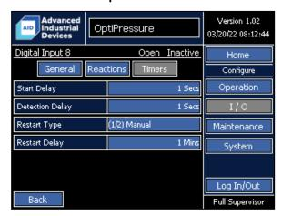
Digital Input 8 does not have a dedicated function and can be used for as a general purpose indicator, an alarm, a shutdown, or any of the functions that allow selection of a digital input for operation — such as the dump valve. The name can be modified by the operator.
