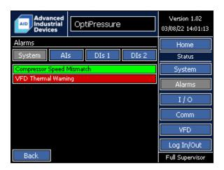
Individual alarm events are listed on the Alarms screen. Alarm events that are not currently present (inactive/OK) are displayed in black text over a green background. When an alarm event is currently present (active), the individual alarm indicator will be displayed in white text over a red background.
