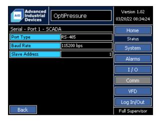
Ethernet communication between the OptiPressure controller and the variable frequency drive is required. Serial communication between the two devices is NOT supported.
