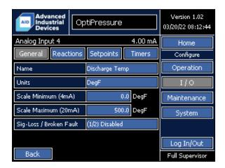
Math conversions for the engineering units are not automatically performed by the controller. Any conversions required to change the units specified on the sensor to a different engineering units scale must be performed by the operator by setting the Units, Scale Minimum (4mA), and Scale Maximum (20mA) parameters.
