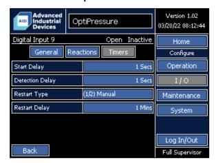
Digital Input 9 does not have a dedicated function and can be used for as a general purpose indicator, an alarm, a shutdown, or any of the functions that allow selection of a digital input for operation — such as the dump valve. The name can be modified by the operator.
