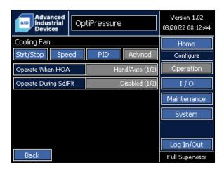
**Cooling Fan – Advanced** parameters are available when **Cooling Fan – Start/Stop > Control Mode** is set to By Temperature. **Cooling Fan – Advanced** parameters are disabled when **Cooling Fan – Start/Stop > Control Mode** is set to Disabled or With Compressor.
