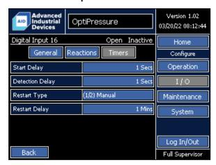
Digital Input 16 does not have a dedicated function and can be used for as a general purpose indicator, an alarm, a shutdown, or any of the functions that allow selection of a digital input for operation — such as the dump valve. The name can be modified by the operator.
