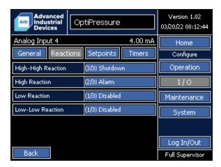
Each analog input supports independent reactions to the four setpoints. The multiple setpoints and reactions provide a flexible method to create warnings/notifications that alert the operator a sensor indicates a high or low condition and if the measured value continues to increase or decrease to the high-high or low-low setpoint, trigger a shutdown event.
