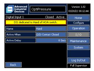
The function of Digital Input 1 is dedicated to the Hand operation of the HOA switch. The name can be modified by the operator.
