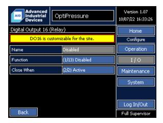
Digital Output 16 is a multipurpose digital output with a function selectable by the operator. The Name automatically changes based on the function selected and cannot be modified by the operator.
