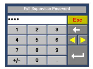
Entering the correct password will result in the display returning to the screen from which the Log In/Out button was pressed. Pressing the Esc button will return to the Log In screen, and pressing the Back button from the Log In screen will also result in the display returning to the screen from which the Log In/Out button was initially pressed.
