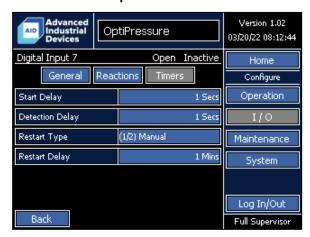
Digital Input 7 does not have a dedicated function and can be used for as a general purpose indicator, an alarm, a shutdown, or any of the functions that allow selection of a digital input for operation — such as the dump valve. The name can be modified by the operator.
