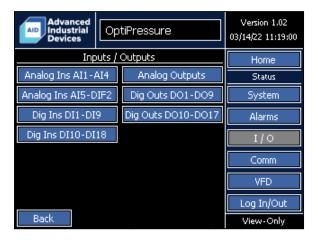
The OptiPressure controller provides a robust set of analog and digital I/O that allows for monitoring and control of a variety of external devices. For operator simplicity, the analog and digital I/O status information is grouped by I/O type.
