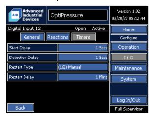
Digital Input 12 does not have a dedicated function and can be used for as a general purpose indicator, an alarm, a shutdown, or any of the functions that allow selection of a digital input for operation — such as the dump valve. The name can be modified by the operator.
