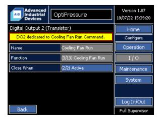
The function of Digital Output 2 is dedicated to the run command of the cooling fan motor starter or variable frequency drive.
