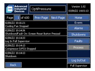
Process events do not record a snapshot at the time the entry is recorded. Since the system is operating normally, the SD card data logging is recommended for tracking performance in this case.
