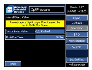
An optional vessel bleed valve can be installed to open a valve while the compressor is stopped to relieve vessel pressure. The valve is closed during normal operation while the compressor is running.
