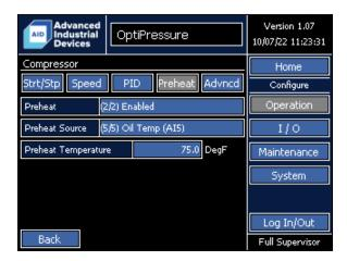
Compressor oil viscosity increase as temperature decreases. Since a seal is created by the oil in rotary screw compressors, the increased oil viscosity at lower temperatures increases wear and reduces the efficiency of the system. Compressor oil preheat runs the compressor at minimum speed during startup until the oil temperature reaches an operator-defined setpoint. Once the oil temperature reaches the setpoint, the controller releases the compressor to run at a speed based on normal operation.
