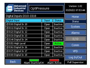
Digital inputs 1 through 9 are shown on the first Digital Inputs I/O status screen and digital inputs 10 through 18 are shown on the second Digital Inputs I/O status screen. Each row in the table represents a single digital input, and provides the following:
