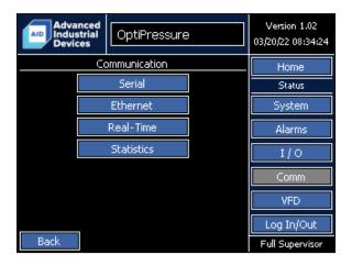
The OptiPressure controller supports several configurable data communication methods. The Communication Status screens summarize all of the communication configuration parameter values and key communication statistics. The availability of all the communication data in a single location provides the operator or technician with quick access to key parameter values needed for commissioning or troubleshooting.
