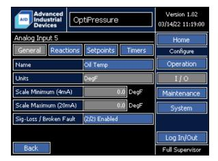
Discharge temperature is the recommended function for Analog Input 5. Both the name and units can be modified by the operator, when configured for a 4-20 mA input. When configured for a K-type thermocouple or 100-ohm platinum RTD, the Units, Scale Minimum, and Scale Maximum cannot be modified.
