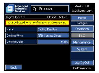
The function of Digital Input 4 is dedicated to the run confirmation of the cooling fan. If a cooling fan is used, either with a motor starter or a variable frequency drive, Digital Input 4 should be connected to a set of dry/unpowered contacts on the motor starter (auxiliary contacts) or drive (relay or transistor output programmed to close when the drive is running).
