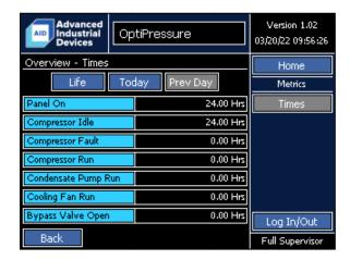
Function time and operational data are tracked on the Metrics Times screen. Metrics data can be used for determining when equipment maintenance should be performed and/or if daily operational performance has been affected by changes to the system.
