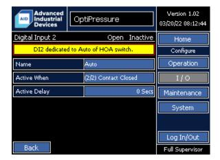
The function of Digital Input 2 is dedicated to the Auto operation of the HOA switch. The name can be modified by the operator.
