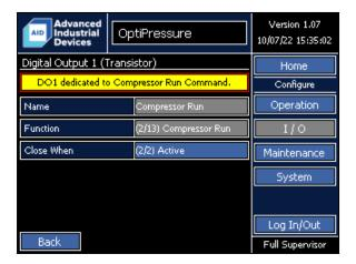
The function of Digital Output 1 is dedicated to the run command of the compressor variable frequency drive. When the OptiPressure controller is used with a Fuji MEGA variable frequency drive, the run command is sent over the Ethernet communication link and Digital Output 1 is not required.
