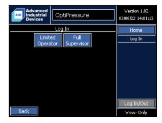
After pressing either of the access level buttons, the operator will be prompted for the password for the selected access level.
