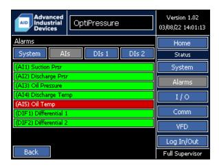
For analog input alarms, the text on the individual alarm indicators will automatically be updated with the names entered by the operator on the configuration screen for the associated input.
