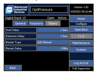
Digital Input 10 does not have a dedicated function and can be used for as a general purpose indicator, an alarm, a shutdown, or any of the functions that allow selection of a digital input for operation — such as the dump valve. The name can be modified by the operator.
