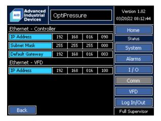
Ethernet communication between the OptiPressure controller and the variable frequency drive is required. Serial communication between the two devices is NOT supported.
