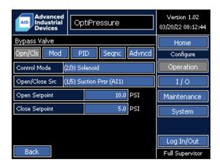
An optional bypass valve can be installed connecting the suction side to the discharge side of the compressor. The function of the bypass valve can vary depending on the type of compressor and site requirements, but is commonly used to unload the compressor during startup or allow the compressor to run at a more optimal speed.
