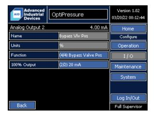
Analog Output 2 is a multipurpose analog output with a function selectable by the operator. The Name and Units automatically change based on the function selected and cannot be modified by the operator.
