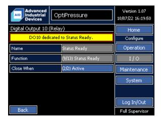
The function of Digital Output 10 is dedicated to the ready status indication of the system. Ready status indication is active when the HOA is in the Hand or Auto position, the system is stopped, and does not have an active shutdown or fault event.
