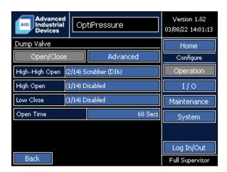
The OptiPressure controller supports several dump valve configurations depending on the number of liquid sensors installed. In all configurations, the high-high shutdown sensor is required, while the high open and low close are sensors are optional.
