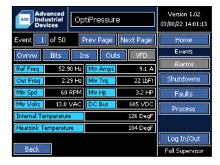
Navigation on the Event Details screen operates similarly to the Event List Screen. The Prev Page and Next Page buttons at the top of the screen move backward and forward one event at a time, displaying the snapshot data
