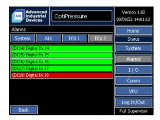
For digital input alarms, the text on the individual alarm indicators will automatically be updated with the names entered by the operator on the configuration screen for the associated input.
