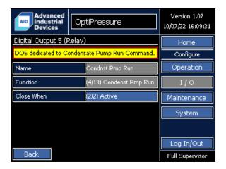
The function of Digital Output 5 is dedicated to the run command of the condensate pump.
