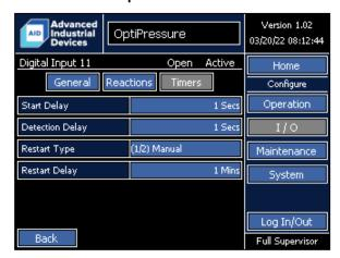
Digital Input 11 does not have a dedicated function and can be used for as a general purpose indicator, an alarm, a shutdown, or any of the functions that allow selection of a digital input for operation — such as the dump valve. The name can be modified by the operator.
