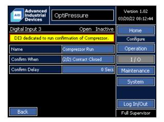
The function of Digital Input 3 is dedicated to the run confirmation of the compressor. When the OptiPressure controller is used with a Fuji MEGA variable frequency drive, the compressor run confirmation is obtained over the Ethernet communication link and Digital Input 3 is not required.
