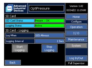
The OptiPressure controller supports a standard SD card, which can be used for periodic data logging, saving/loading configuration parameter values, and upgrading the controller firmware. The SD card MUST be specially formatted in order for the controller to properly recognize and use the SD card. Refer to the **SD Card Formatting** section for more detailed information on this process.
