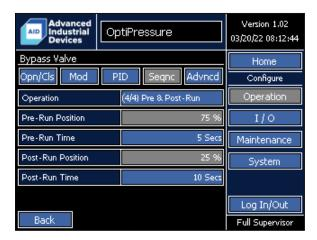
The bypass valve can be configured to open for a set duration as part of the Pre-Run and/or Post-Run sequence of the compressor. This overrides the **Bypass Valve – Open/Close > Open Setpoint**, and immediately commands the bypass valve to open. The bypass valve will close again only when the **Bypass Valve – Open/Close > Close Setpoint** condition is met.
