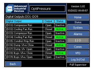
Digital outputs 1 through 9 are shown on the first Digital Outputs I/O status screen. The Digital Outputs status screen presents information in a similar layout to the Digital Inputs status screen. The key difference is the digital outputs do not have alarm indications, as the outputs cannot be configured for alarm or shutdown events. Each row in the table represents a single digital output, and provides the following information:
