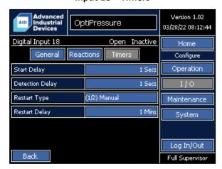
Digital Input 18 does not have a dedicated function and can be used for as a general purpose indicator, an alarm, a shutdown, or any of the functions that allow selection of a digital input for operation — such as the dump valve. The name can be modified by the operator.
