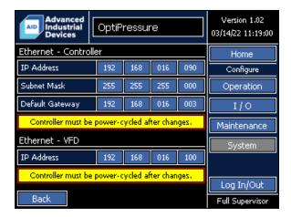
The OptiPressure controller supports two external device communication ports. The Ethernet port provides communication with both the variable frequency drive and with SCADA devices. One serial port is dedicated to communication with SCADA devices.
