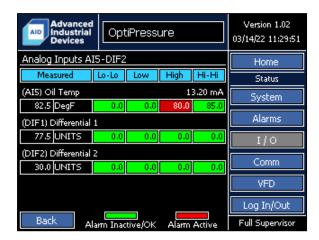
Analog inputs 1 through 4 are shown on the first Analog Inputs I/O status screen and analog inputs 5 through DIF2 are shown on the second Analog Inputs I/O status screen. Each row in the table represents a single analog input, and provides the following:
