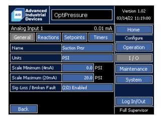
Suction pressure is the recommended function for Analog Input 1. Both the name and units can be modified by the operator.
