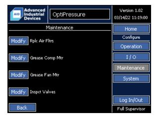
The OptiPressure controller includes a built-in Maintenance Reminder system that can automatically remind operators of the need to perform maintenance and other tasks at set intervals. Four customizable Maintenance Reminders are available, each with independent reminder conditions.
