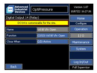
Digital Output 14 is a multipurpose digital output with a function selectable by the operator. The Name automatically changes based on the function selected and cannot be modified by the operator.
