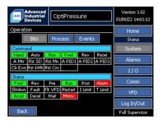
Command and Status bits are duplicated on both the System Operation and System Performance status groups in order to provide a quick reference for the local operator, without the need to flip back and forth between groups for the needed information.
