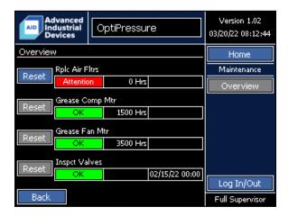
The OptiPressure controller includes a built-in Maintenance Reminder system that can automatically remind operators of the need to perform maintenance and other tasks at set intervals. When one or more of the Maintenance Reminders becomes active, a notification appears on the Home screen, a Modbus SCADA indication bit is set, and a Process event entry is recorded.
