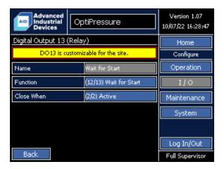
Digital Output 13 is a multipurpose digital output with a function selectable by the operator. The Name automatically changes based on the function selected and cannot be modified by the operator.
