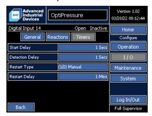
Digital Input 14 does not have a dedicated function and can be used for as a general purpose indicator, an alarm, a shutdown, or any of the functions that allow selection of a digital input for operation — such as the dump valve. The name can be modified by the operator.
