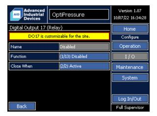
Digital Output 17 is a multipurpose digital output with a function selectable by the operator. The Name automatically changes based on the function selected and cannot be modified by the operator.
