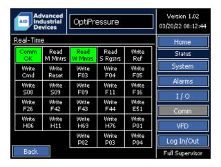
Stable, reliable Ethernet communication between the OptiPressure controller and the variable frequency drive is a critical component to the optimal performance of the system as a whole. Since unknown site conditions may affect the quality of the communications link at the time of installation or later when site conditions change, the Communication Status screens provide capture of communication error messages, if errors occur.
