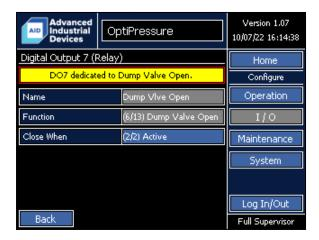
The function of Digital Output 7 is dedicated to the open command of the dump valve.
