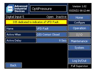
The function of Digital Input 5 is dedicated indication of a fault condition of the variable frequency drive. When the OptiPressure controller is used with a Fuji MEGA variable frequency drive, the drive fault status is obtained over the Ethernet communication link and Digital Input 5 is not required.
