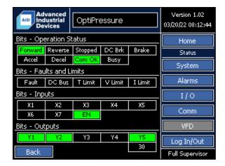
The status indicators and monitor values displayed on the Variable Frequency Drive Status screen are the values read directly from the variable frequency drive monitor registers. The values are unmodified or manipulated, and can be used for troubleshooting when checking to verify that the information being presented by the variable frequency drive to the controller for decision-making are expected and/or sensible values.
