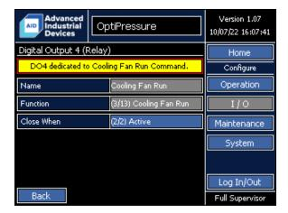
The function of Digital Output 4 is dedicated to the run command of the cooling fan motor starter or variable frequency drive.
