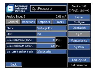
Discharge pressure is the recommended function for Analog Input 2. Both the name and units can be modified by the operator.
