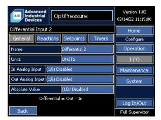
The analog differential input is based on two sensors. The operator must select a combination of two sensors to enable this feature. The analog differential input is calculated by subtracting the Outlet Analog Input from the Inlet Analog Input.
