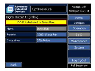
The function of Digital Output 11 is dedicated to the run status indication of the system. Run status indication is active when the system is in the Pre-Run, Run, or Post-Run sequence. The output toggles (blinks) when in the Pre-Run and Post-Run sequences. The output is solid (steady) when in the Run sequence.
