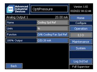
Analog Output 1 is a multipurpose analog output with a function selectable by the operator. The Name and Units automatically change based on the function selected and cannot be modified by the operator.
