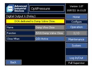
The function of Digital Output 6 is dedicated to the close command of the dump valve.
