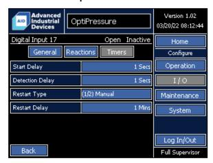
Digital Input 17 does not have a dedicated function and can be used for as a general purpose indicator, an alarm, a shutdown, or any of the functions that allow selection of a digital input for operation — such as the dump valve. The name can be modified by the operator.
