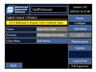
The function of Digital Output 9 is dedicated to the open command of the bypass valve.
