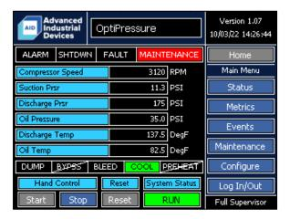
The Home screen provides an overview of the operational values of the compressor system, and is used as the launching point for navigating to more advanced features of the controller, such as configuration and diagnostic information.
