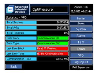
If a communication error does occur, the communication block that experiences the problem will be shown in the Error Block monitor and the type of communication error shown in the Error Type monitor. Once the communication error has been resolved, the values of Error Block and Error Type are moved to the Last Error Block and Last Error Type monitors, to provide some historical information if the communication error occurs only intermittently.
