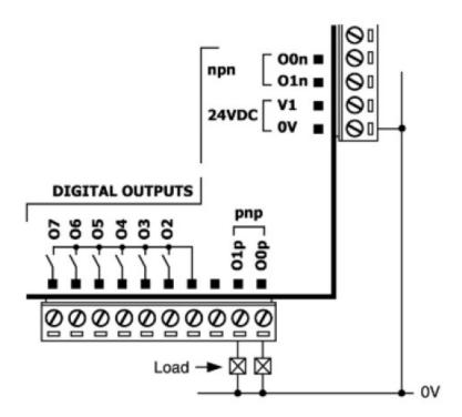
Each of the two groups of **RELAY** digital outputs (O2 through O16 on the diagram below) has a common connection to the relay bank.
