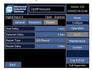
Digital Input 6 does not have a dedicated function and can be used for as a general purpose indicator, an alarm, a shutdown, or any of the functions that allow selection of a digital input for operation — such as the dump valve. The name can be modified by the operator.
