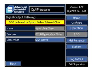
The function of Digital Output 8 is dedicated to the close command of the bypass valve.
