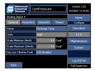
Discharge temperature is the recommended function for Analog Input 4. Both the name and units can be modified by the operator, when configured for a 4-20 mA input. When configured for a K-type thermocouple or 100-ohm platinum RTD, the Units, Scale Minimum, and Scale Maximum cannot be modified.
