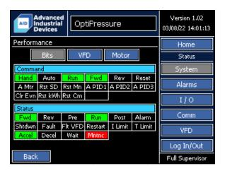
Command and Status bits are duplicated on both the System Operation and System Performance status screens in order to provide a quick reference for the local operator, without the need to flip back and forth between screens for the needed information.
