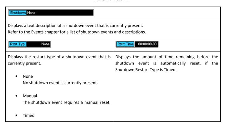
The shutdown event will automatically reset when the Shutdown Restart Time elapses. The shutdown event can also be manually reset before the Shutdown Restart Time elapses.
