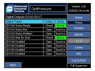
Digital outputs 10 through 17 are shown on the first Digital Outputs I/O status screen. The Digital Outputs status screen presents information in a similar layout to the Digital Inputs status screen. The key difference is the digital outputs do not have alarm indications, as the outputs cannot be configured for alarm or shutdown events. Each row in the table represents a single digital output, and provides the following information:
