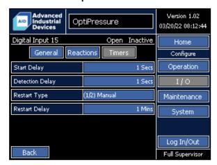
Digital Input 15 does not have a dedicated function and can be used for as a general purpose indicator, an alarm, a shutdown, or any of the functions that allow selection of a digital input for operation — such as the dump valve. The name can be modified by the operator.
