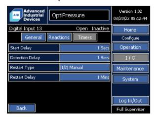
Digital Input 13 does not have a dedicated function and can be used for as a general purpose indicator, an alarm, a shutdown, or any of the functions that allow selection of a digital input for operation — such as the dump valve. The name can be modified by the operator.
