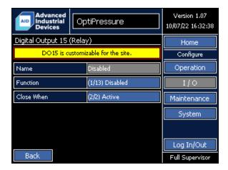
Digital Output 15 is a multipurpose digital output with a function selectable by the operator. The Name automatically changes based on the function selected and cannot be modified by the operator.
