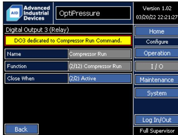
The function of Digital Output 3 is dedicated to the run command of the compressor variable frequency drive. When the OptiPressure controller is used with a Fuji MEGA variable frequency drive, the run command is sent over the Ethernet communication link and Digital Output 1 is not required.
