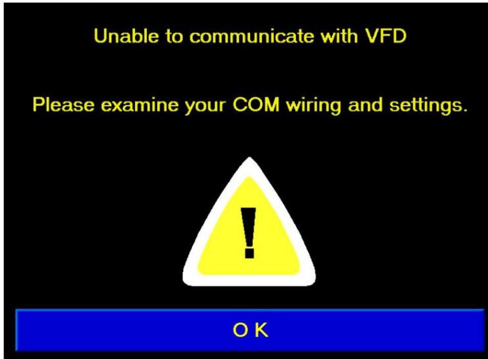
**COM Lost:** This indicates a communications failure between the controller and the VFD.
